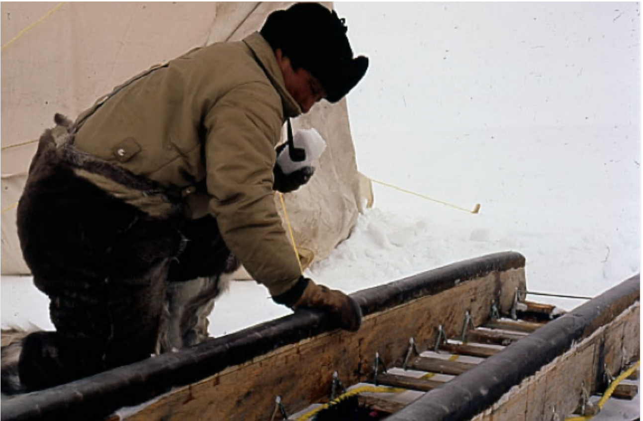
Mud sled runners slicked with freezing water to create 'ice-on-ice' runners that are totally frictionless (Colin Irwin — Arctic Trek 1973)
